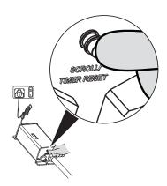
Hold down the timer reset button and reapply power to the controller until you see  $\lceil -5 \rceil = \lceil -5 \rceil$ , then release timer reset button. A 5 second delay will occur until you hear an audible tone and LED display will read once again  $\lceil -3 \rceil = \lceil -5 \rceil$ .
