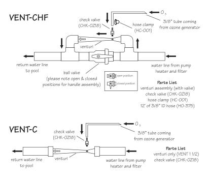
Figure 3 Water Venturi System
