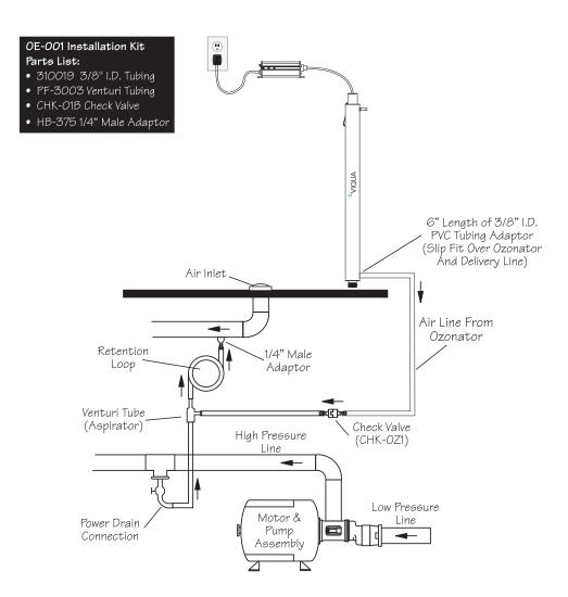
Figure 2 Pressure Differential System
